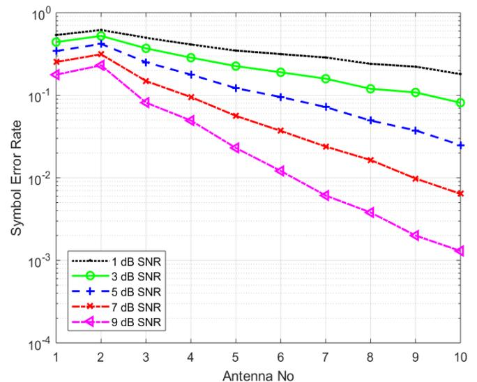
Figure 5: SER versus antenna numbers in array
