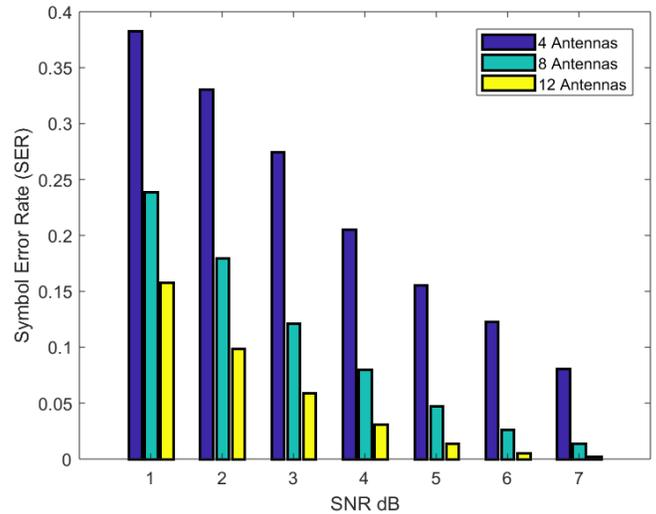
Figure 4: SER comparison of different number of antenna arrays
