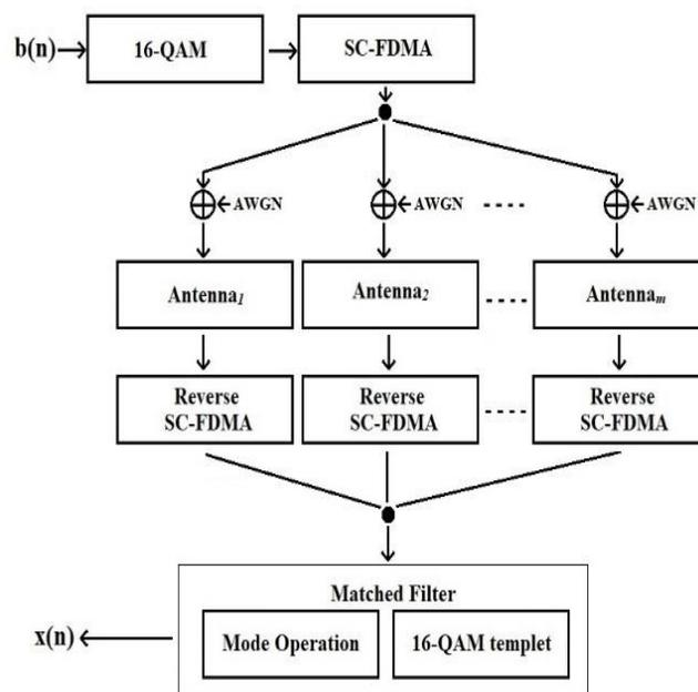
Figure 2: Uplink of Massive MIMO System Model
